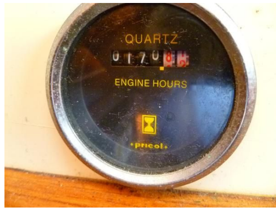
Engine hours run meter.
