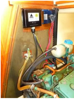
Engine bay showing battery charging regulator
